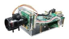
The brand new megapixel CMOS ISP, EAGLET2 Series (NVP2440H/2441H) has state-of-the art technology to give the finest image quality. Especially it is designed to meet the demands of new trends in CCTV market, both Analog FHD Camera and cost-effective HD-SDI applications. EAGLET2 series is supporting 2.0M CMOS sensor and output I/F as digital(1080p) and analog AHD2.0/CVBS/COMET.
