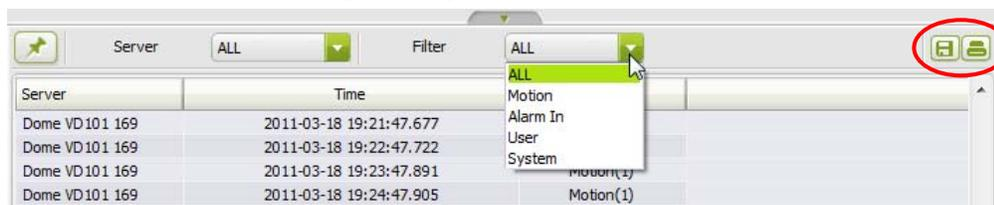
Those event log messages can be saved as a file or printed out by clicking related buttons on top right of event log window. (Max. 1,000 log messages (100 messages for Lite version) can be saved into \*.csv file format)
